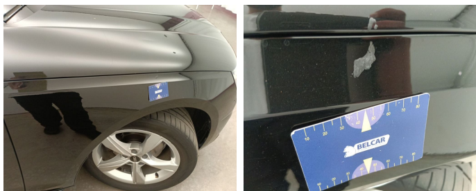
Wing Front right // Painting-Chemical reaction
