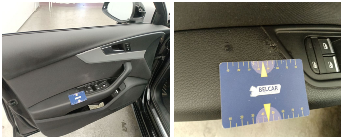
Front Left Door Interior Coating // Replace Completely-Incinerated
