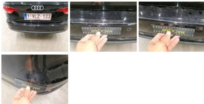
Rear light L, Scratch(es), Acceptable
