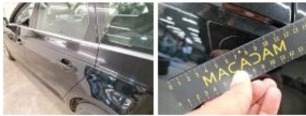
Wing RL, Dent(s), Acceptable
