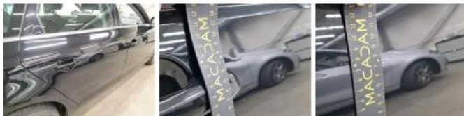
Door FR, Dent(s), Paintless dent repair
