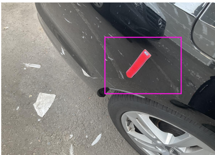
11. Side Panel / Back Right Paint / Scratch / Scuff -
