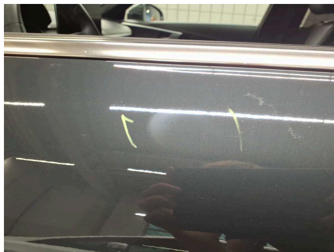
Damage 4: Body: Body - Scratch(es) - Conditioning
