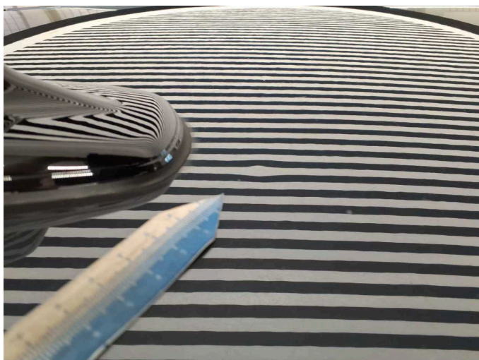
Damage 2: Roof: Roof - dent(s) - Smart repair
