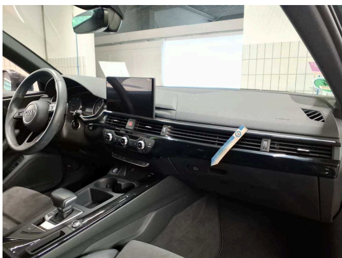
Damage 5: Instrument panel: Cover - Scratch(es) - Replace
