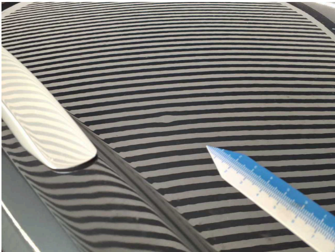
Damage 2: Roof: Roof - dent(s) - Smart repair
