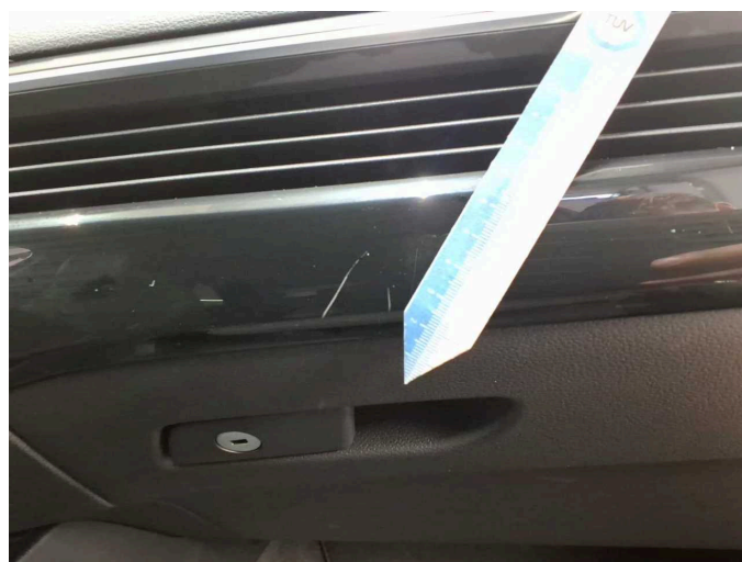
Damage 5: Instrument panel: Cover - Scratch(es) - Replace
