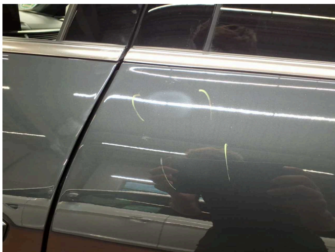
Damage 4: Body: Body - Scratch(es) - Conditioning
