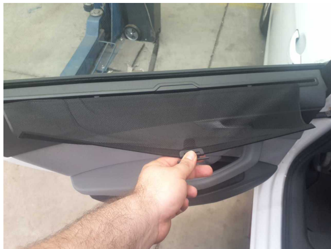
Damage 3: Cab: Sun visor (Tür hinten links) - Deformed - Replace
