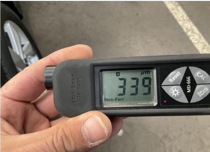
1. Hood Paint / Poor Previous Repair -
