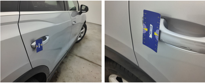
Door Rear Right // Smart Repair Medium-scratch
