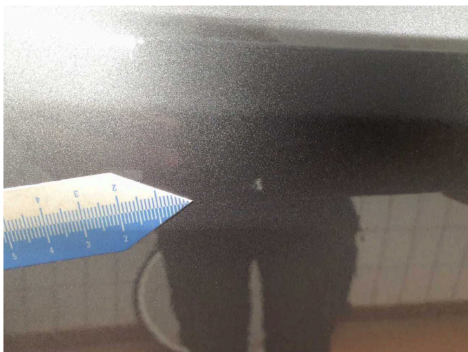
Gebrauchsspur 4: Tür hinten rechts: Tür - Delle / Lackschaden - Smart Repair
