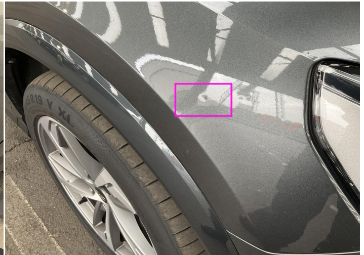
2. Fender / Front Right Bodywork / Dent / Dent -
