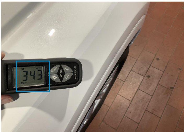
11. Fender / Front Right Paint / Poor Previous Repair -
