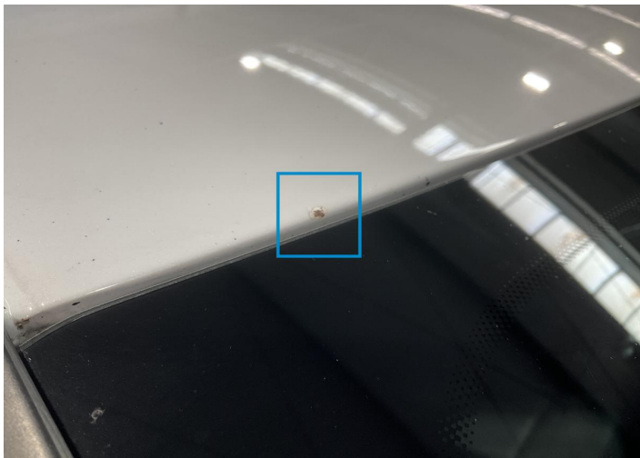
9. Roof Paint / Stone Chip -
