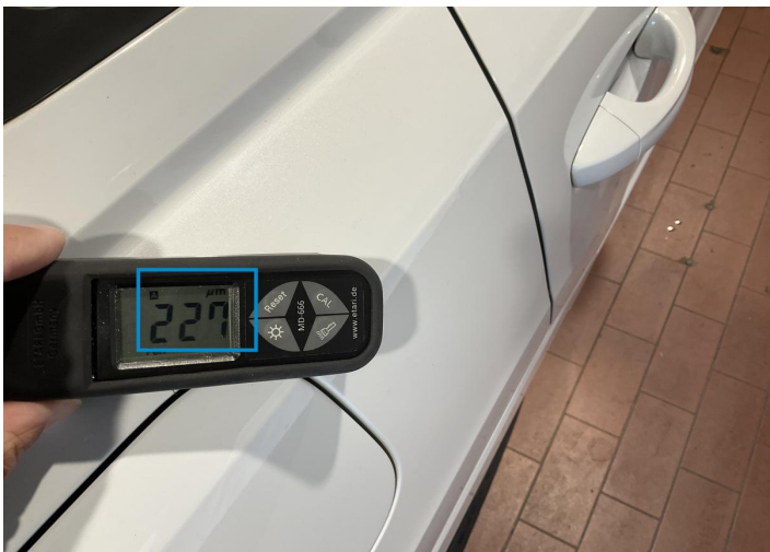
12. Side Panel / Back Right Paint / Poor Previous Repair -
