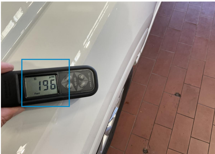
10. Fender / Front Left Paint / Poor Previous Repair -
