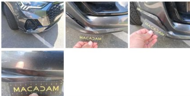
Grille, Broken, Replace
