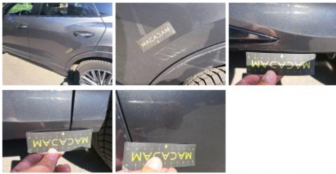
Wing trim RL, Scratch(es), Repair and paint (complete)
