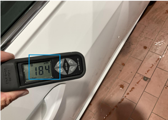
4. Door / Front Right Paint / Poor Previous Repair -
