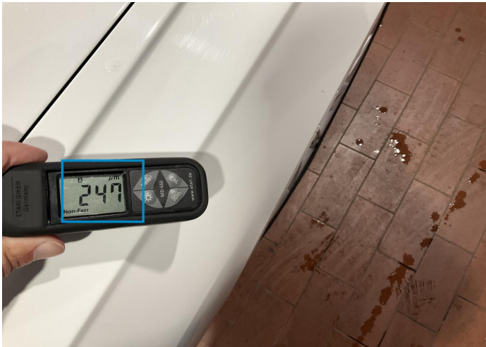
3. Fender / Front Right Paint / Poor Previous Repair -
