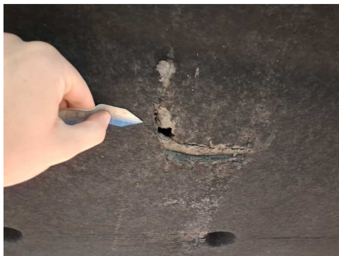
Damage 6: Body: Underbody panelling - Broken / torn - Replace
