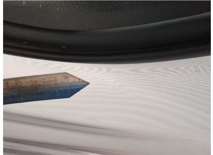
Damage 3: Sill - left side: Sill (+ Aufkleber Reifendruck) - Dent / paintcoat damage - Smart repair
