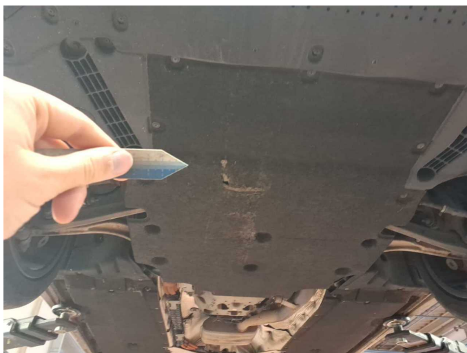
Damage 6: Body: Underbody panelling - Broken / torn - Replace
