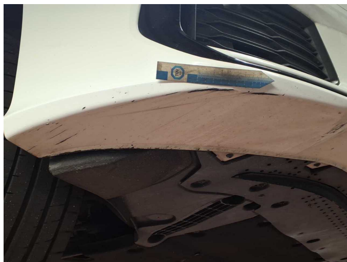
Damage 7: Front bumper: Front bumper (Unterhalb) - Scratched - Paint
