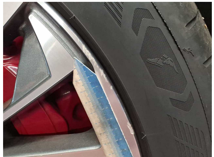
Damage 4: Wheel / tyres: Alloy rim - front left side (Materialabtrag, Optischer Mangel) - Scratched - Loss in value
