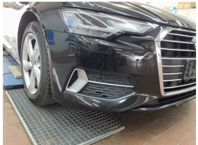
Damage 6: Front bumper: Front bumper - Scratch(es) - Paint
