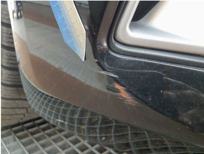
Damage 6: Front bumper: Front bumper - Scratch(es) - Paint
