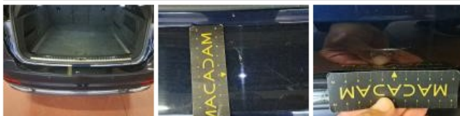
Bumper moulding R, Broken, Replace
