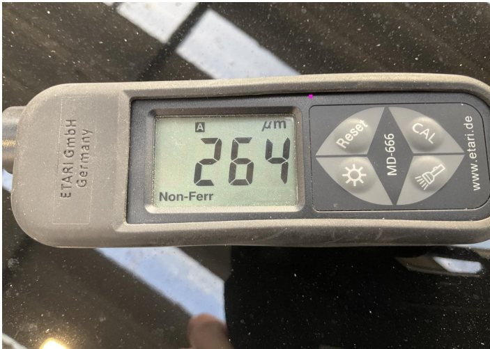
1. Fender / Front Left Paint / Poor Previous Repair -
