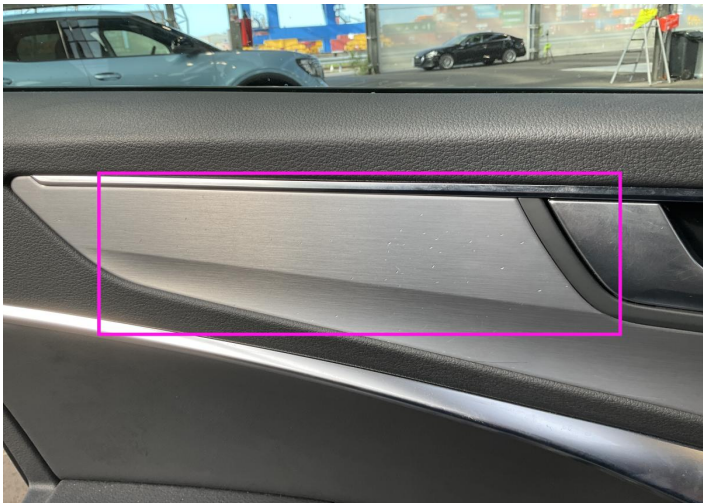
5. Panel Filling / Front Left Interior / Scratched -
