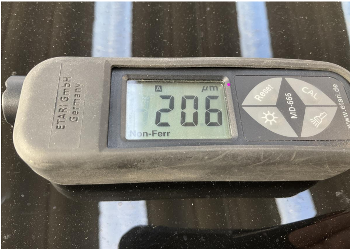
2. Fender / Front Right Paint / Poor Previous Repair -
