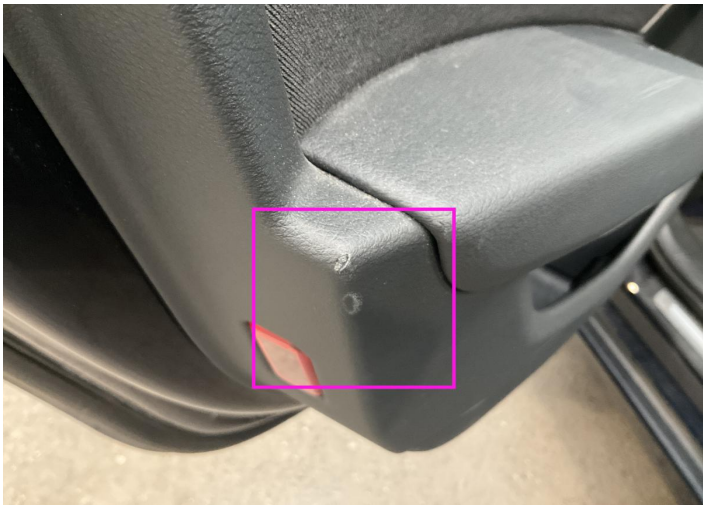
5. Panel Filling / Back Left Interior / Holed -
