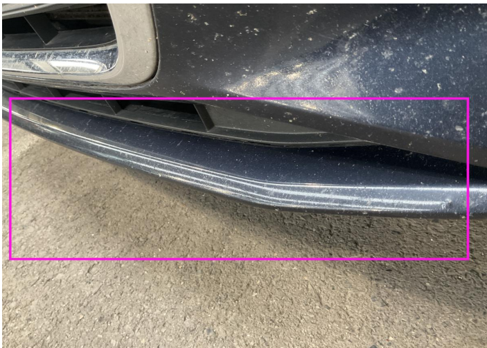
1. Bumper / Front Bodywork / Breakage / Crack -
