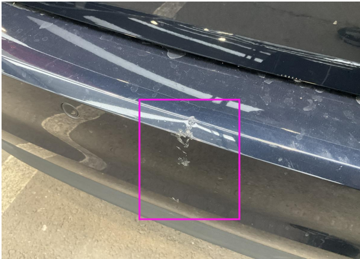
4. Bumper / Back Bodywork / Breakage / Crack -
