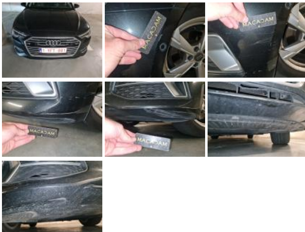
Bumper F, Scratch(es), Repair and paint (complete)
