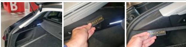
Internal boot lining R, Scratch(es), Acceptable
