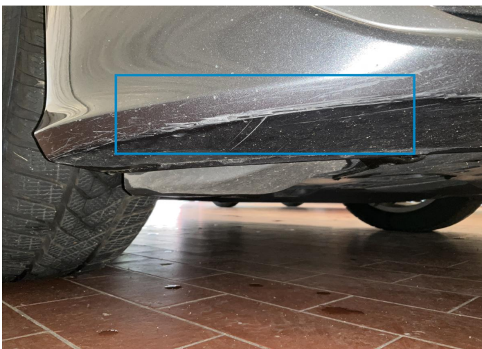
2. Bumper / Front Paint / Scratch / Scuff -
