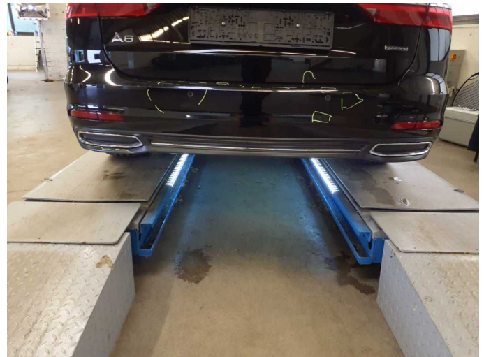
Damage 10: Rear bumper: Spoiler - Scratched - Replace
