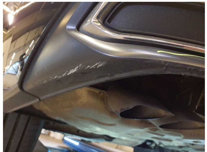
Damage 10: Rear bumper: Spoiler - Scratched - Replace
