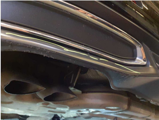
Damage 10: Rear bumper: Spoiler - Scratched - Replace
