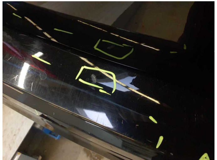
Damage 12: Rear bumper: Rear bumper - Scratched - Paint
