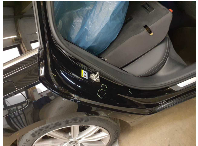
Damage 2: Trim / covers: C-pillar - trim - interior, right side - Scratched - Loss in value
