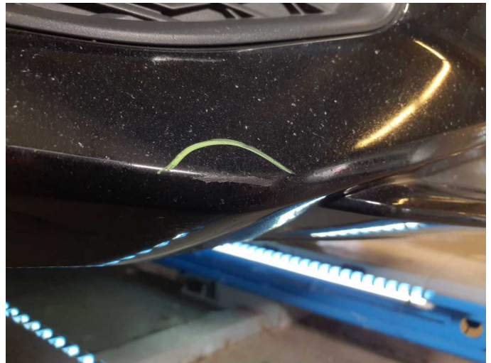
Damage 11: Front bumper: Front bumper - Scratched - Paint
