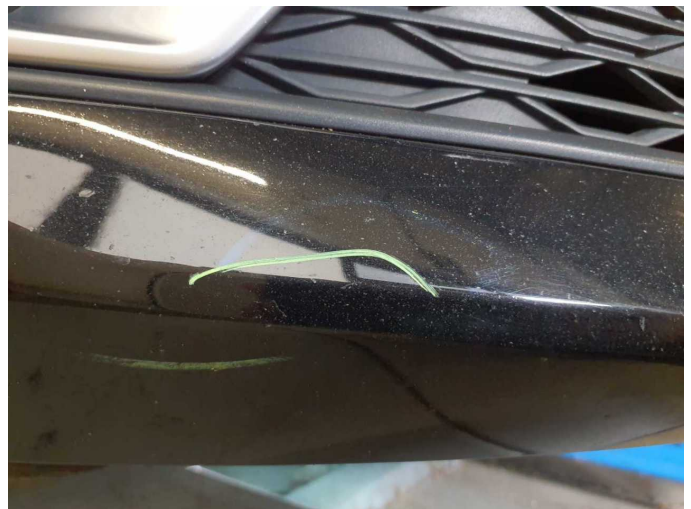
Damage 11: Front bumper: Front bumper - Scratched - Paint
