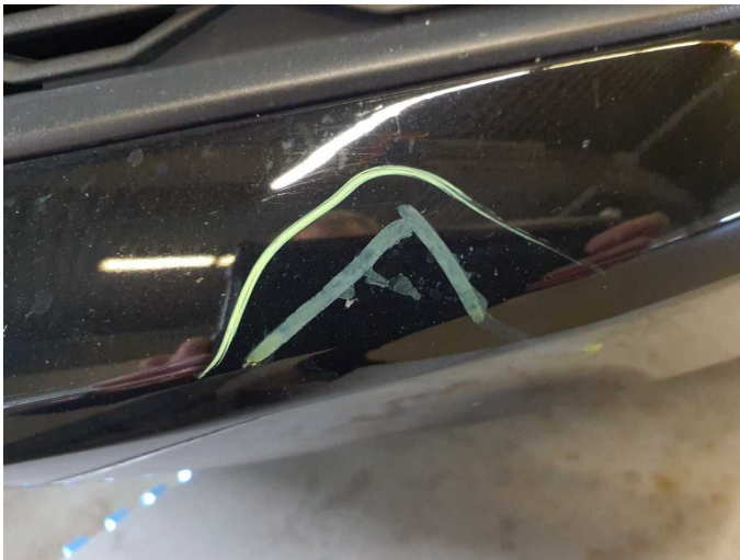
Damage 11: Front bumper: Front bumper - Scratched - Paint
