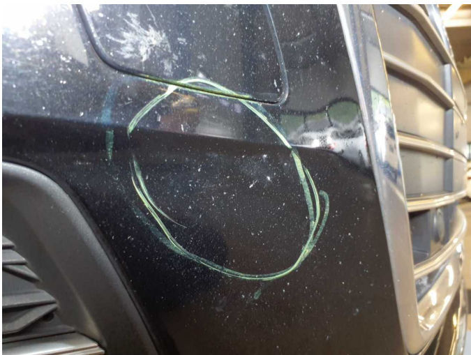
Damage 11: Front bumper: Front bumper - Scratched - Paint
