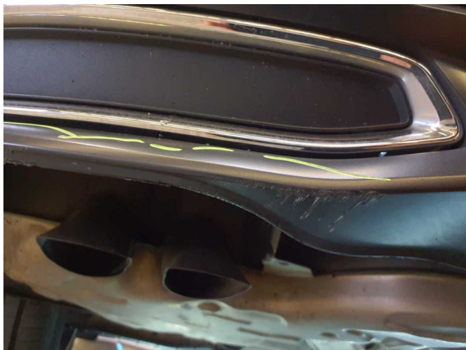
Damage 10: Rear bumper: Spoiler - Scratched - Replace
