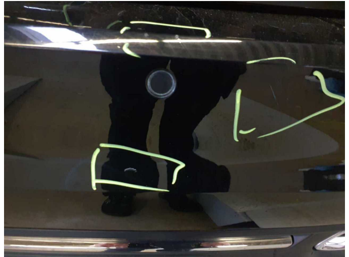
Damage 12: Rear bumper: Rear bumper - Scratched - Paint
