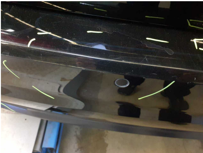
Damage 12: Rear bumper: Rear bumper - Scratched - Paint
