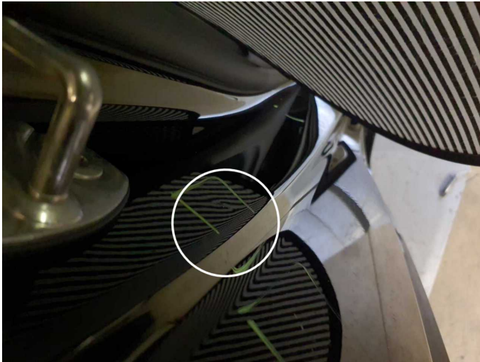
Damage 7: Side panel - rear right side: Sill - Dent / paintcoat damage - Smart repair
