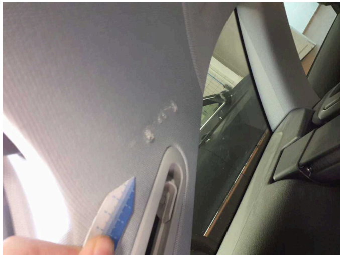
Damage 3: Trim / covers: D-pillar trim - interior, left side - Scratched - Replace
