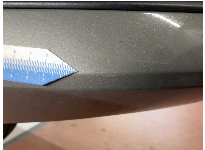
Damage 5: Front bumper: Front bumper - Scratch(es) - Paint
