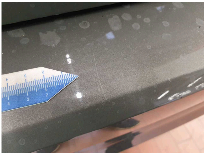
Damage 4: Rear bumper: Rear bumper - Scratch(es) - Paint
