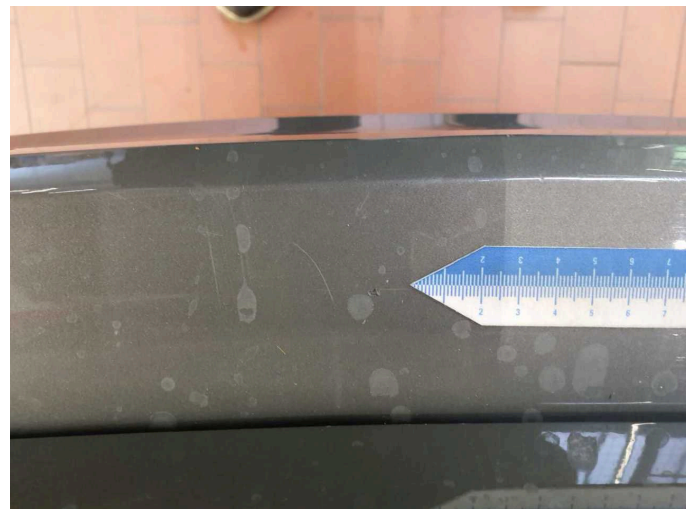
Damage 4: Rear bumper: Rear bumper - Scratch(es) - Paint
