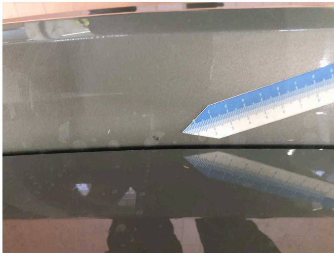
Damage 4: Rear bumper: Rear bumper - Scratch(es) - Paint
