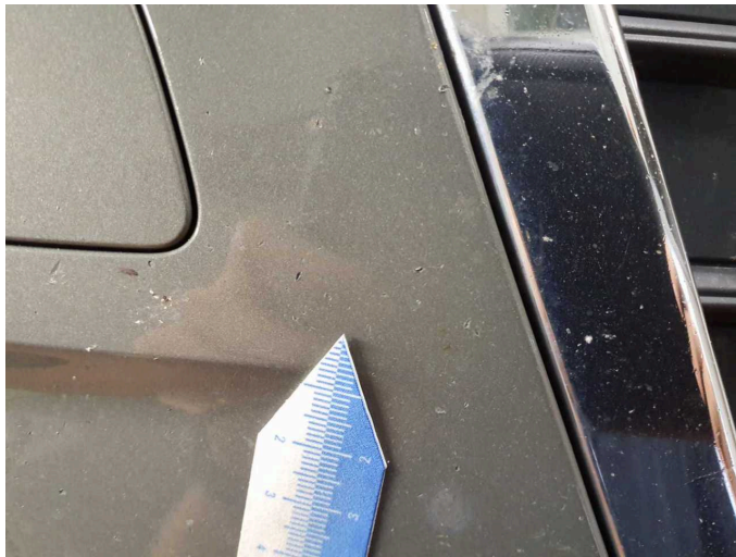
Damage 5: Front bumper: Front bumper - Scratch(es) - Paint
