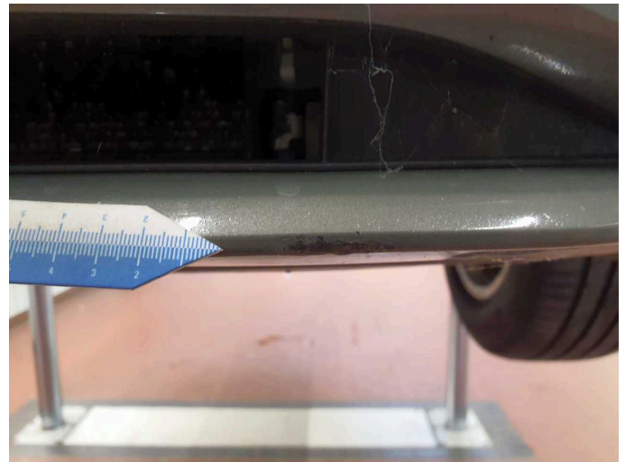
Damage 5: Front bumper: Front bumper - Scratch(es) - Paint
