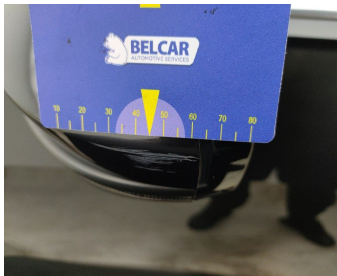
Side View Mirror Left // Painting-scratch
