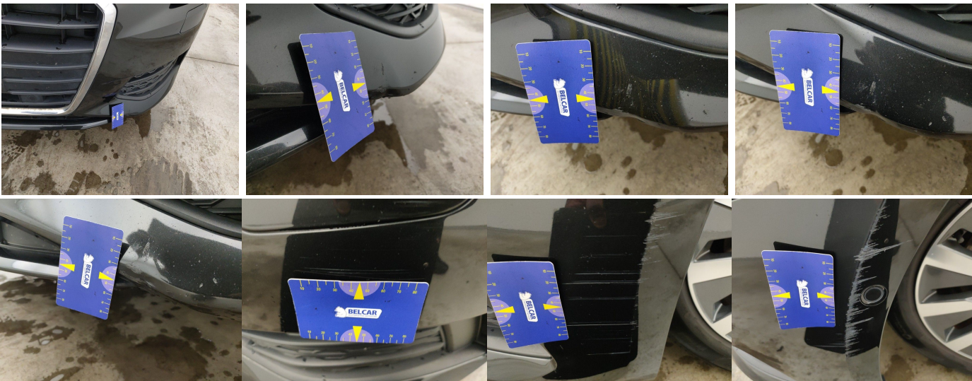
Bumper Front // Repair & Painting-scratch + dent
