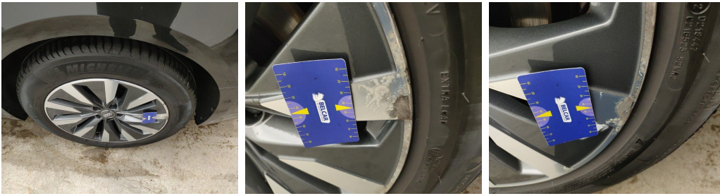
Wheel Two Tone Rear Left // Repair-Chemical reaction
