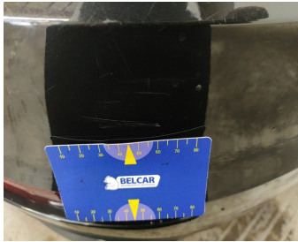
Side View Mirror Left // Painting-scratch
