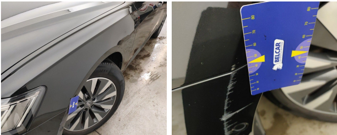
Wing Front Left // Smart Repair Medium-scratch
