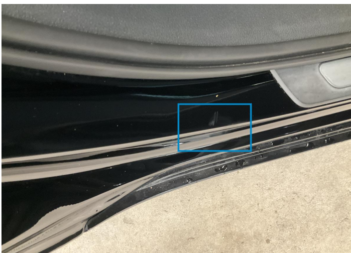
8. Pillar / Back Right Paint / Scratch / Scuff -
