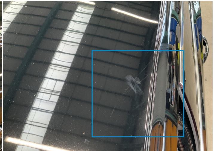
4. Roof Paint / Scratch / Scuff -
