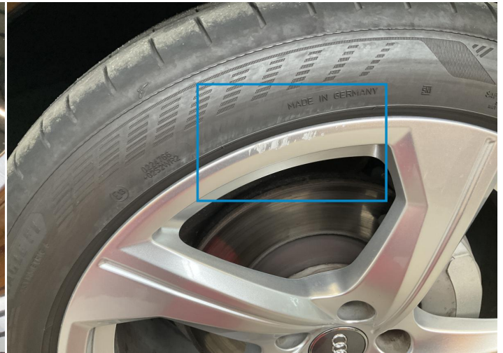
2. Rim / Front Left Out of Bodywork / Scratch -
