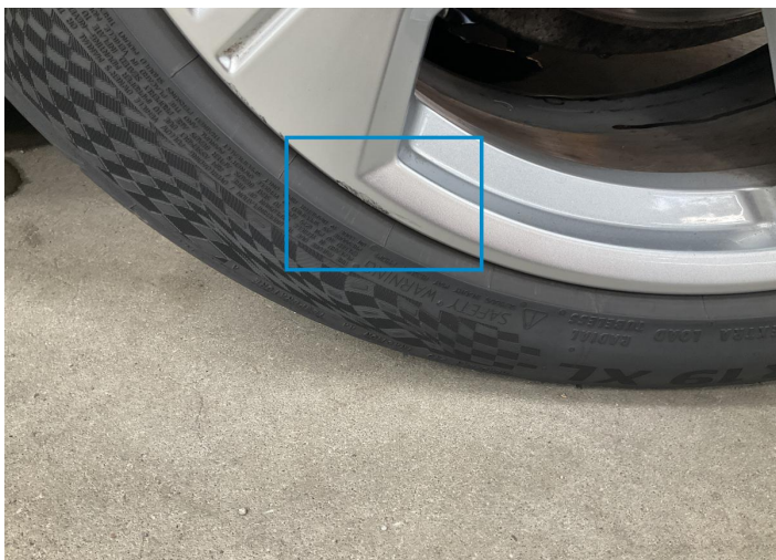
9. Rim / Front Right Out of Bodywork / Scratch -
