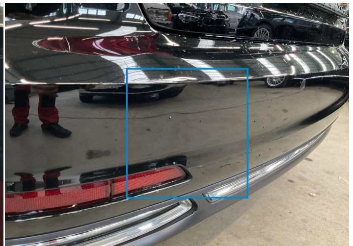
6. Bumper / Back Bodywork / Dent / Dent -
