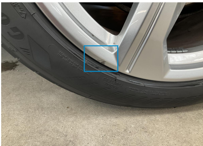
7. Rim / Back Right Out of Bodywork / Scratch -
