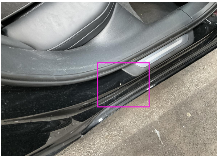
11. Rocker Panel / Center Right Bodywork / Dent / Dent -
