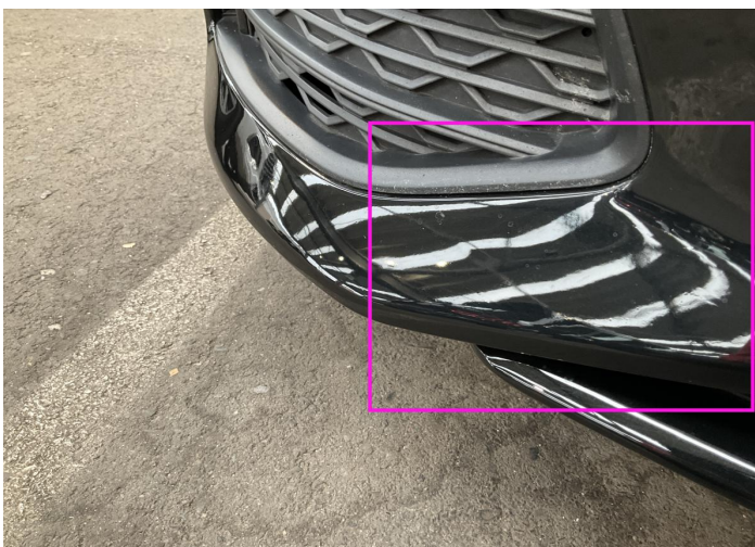
2. Bumper / Front Paint / Poor Previous Repair -
