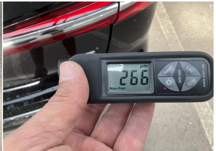
2. Tailgate Paint / Poor Previous Repair -
