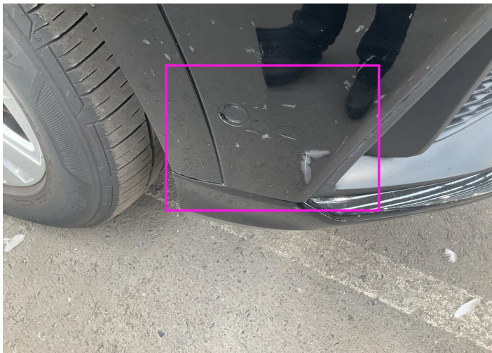
3. Bumper / Front Paint / Scratch / Scuff -
