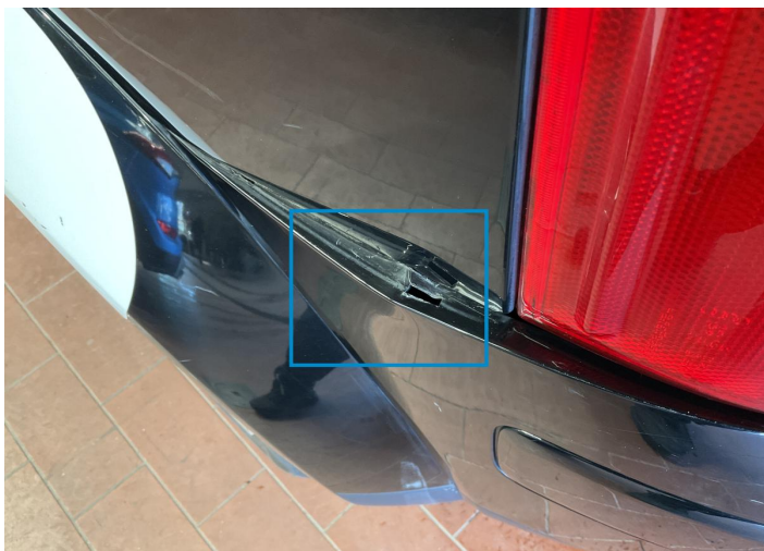
3. Bumper / Back Bodywork / Breakage / Hole -
