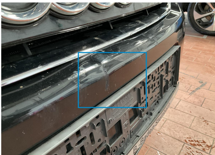
11. Bumper / Front Bodywork / Breakage / Hole -
