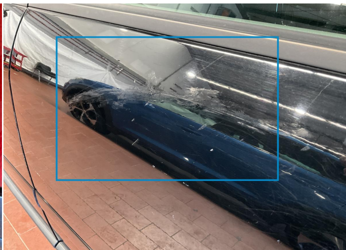
4. Door / Back Left Paint / Poor Previous Repair -
