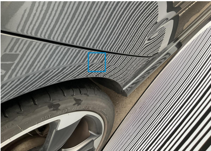
6. Side Panel / Back Right Bodywork / Dent / Dent -
