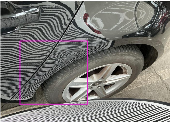
18. Fender / Back Left Bodywork / Dent / Dent -
