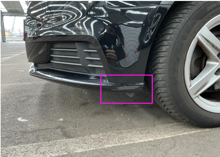
4. Bumper / Front Paint / Scratch / Scuff -
