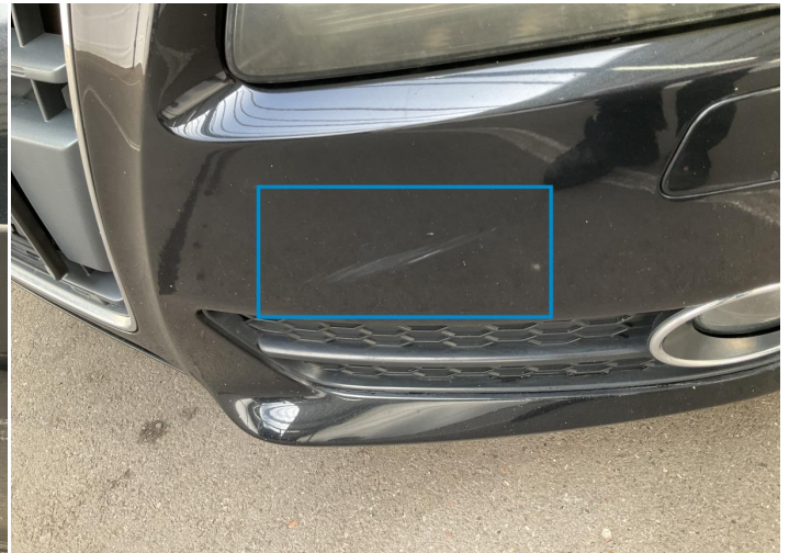
8. Bumper / Front Paint / Scratch / Scuff -
