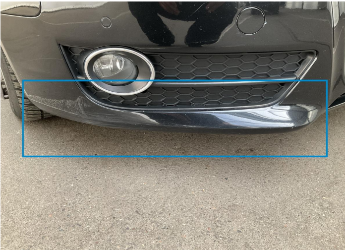
9. Bumper / Front Paint / Scratch / Scuff -
