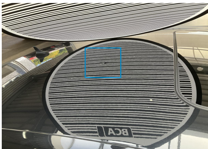
13. Roof Bodywork / Dent / Dent -
