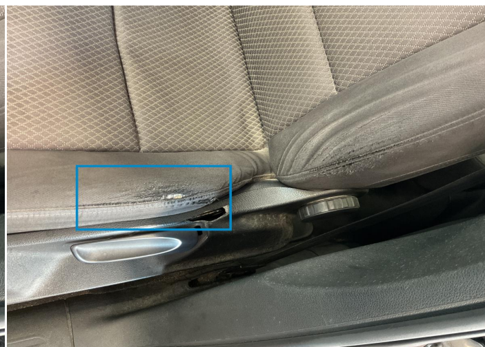
2. Seat / Front Left Interior / Ripped -
