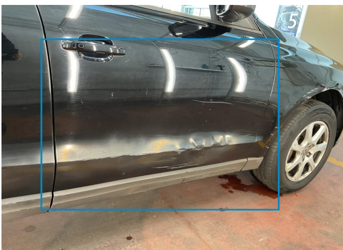
26. Door / Front Right Bodywork / Dent -
