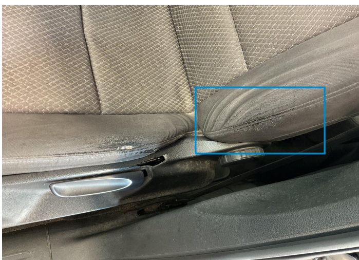
3. Seat / Front Left Interior / Ripped -
