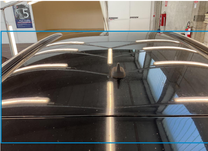
31. Roof Bodywork / Dent / Hail Area -
