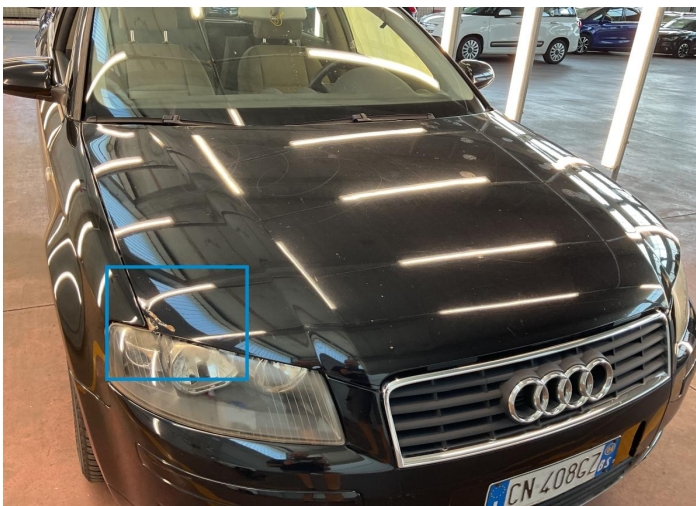
10. Hood Bodywork / Dent -
