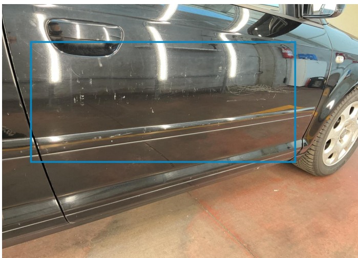
23. Door / Front Right Bodywork / Dent -
