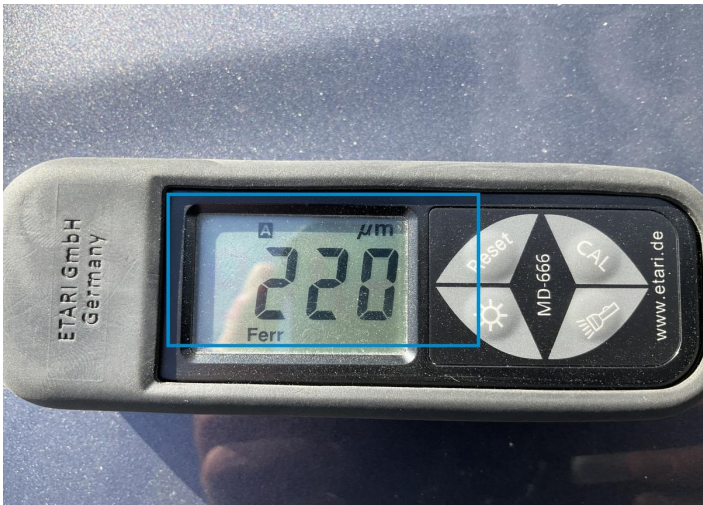
5. Paint / Poor Previous Repair -
