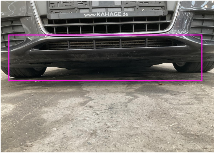
6. Bumper / Front Paint / Scratch / Scuff -
