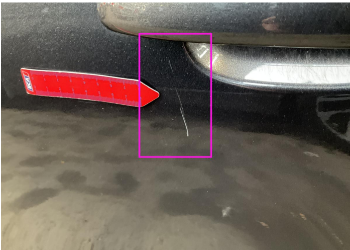
14. Door / Back Left Paint / Scratch / Scuff -
