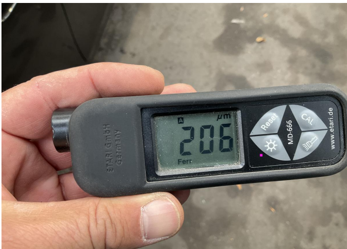
24. Door / Front Left Paint / Poor Previous Repair -
