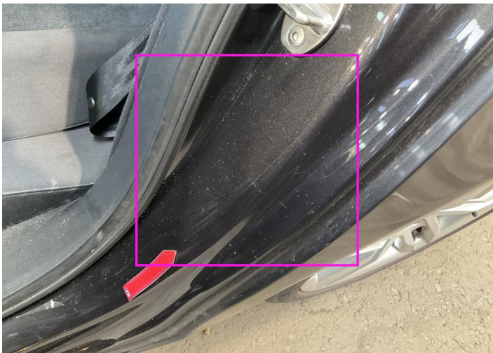
7. Pillar / Back Left Paint / Scratch / Scuff -
