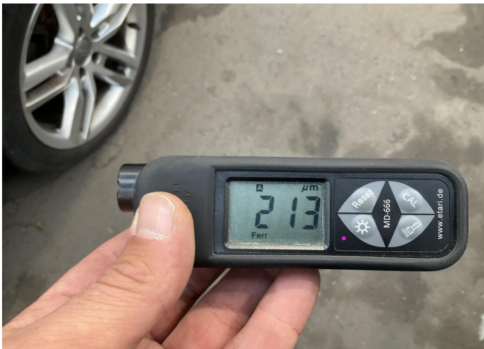
25. Door / Back Left Paint / Poor Previous Repair -
