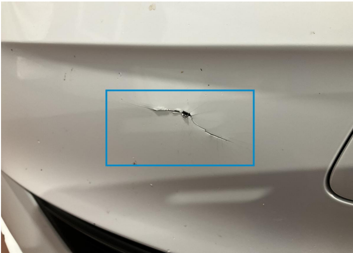
4. Bumper / Front Bodywork / Breakage / Hole -
