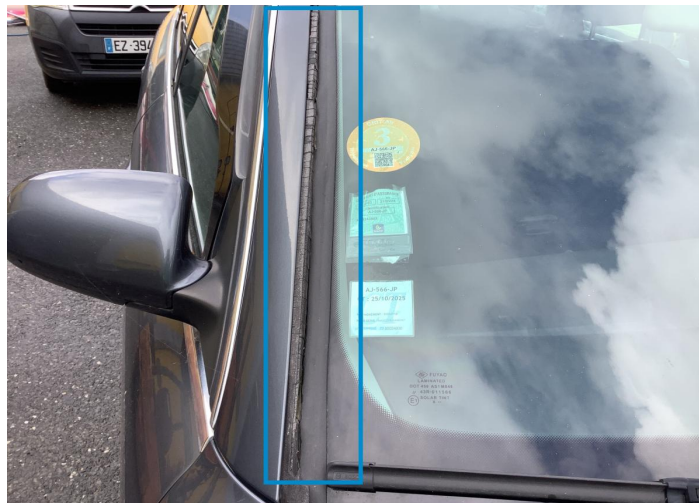
31. Windshield Joint / Front Paint / Chemical Damage -
