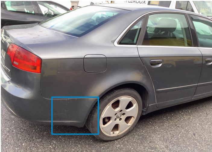
15. Side Panel / Back Right Paint / Scratch / Scuff -
