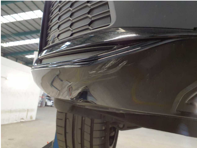
Damage 9: Front bumper: Front bumper - Scratched - Paint
