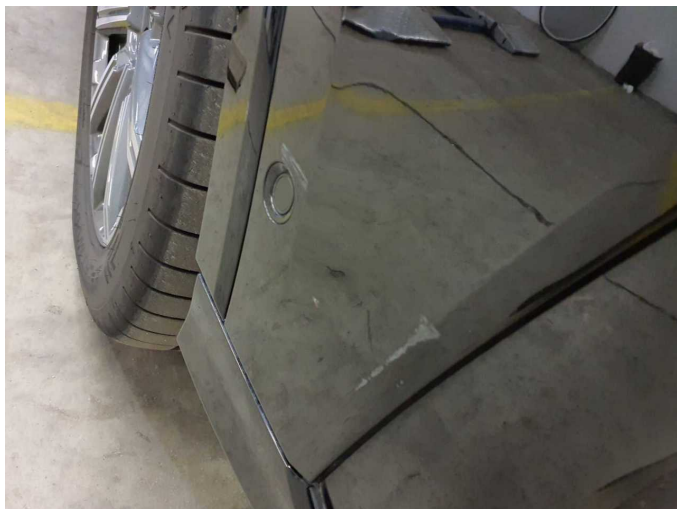
Damage 9: Front bumper: Front bumper - Scratched - Paint
