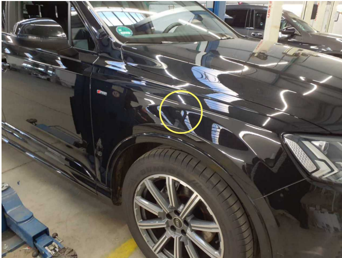
Damage 2: Mudguard - right side: Mudguard - right side - Scratch(es) - Paint
