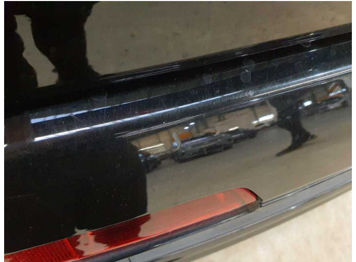
Damage 5: Rear bumper: Rear bumper - Scratch(es) - Paint
