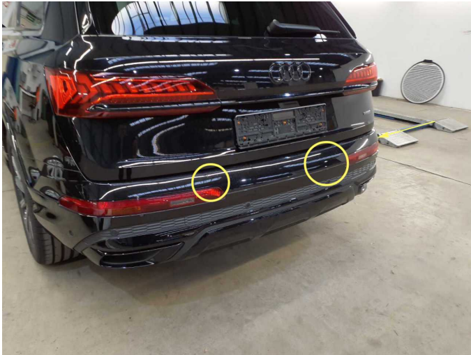
Damage 5: Rear bumper: Rear bumper - Scratch(es) - Paint
