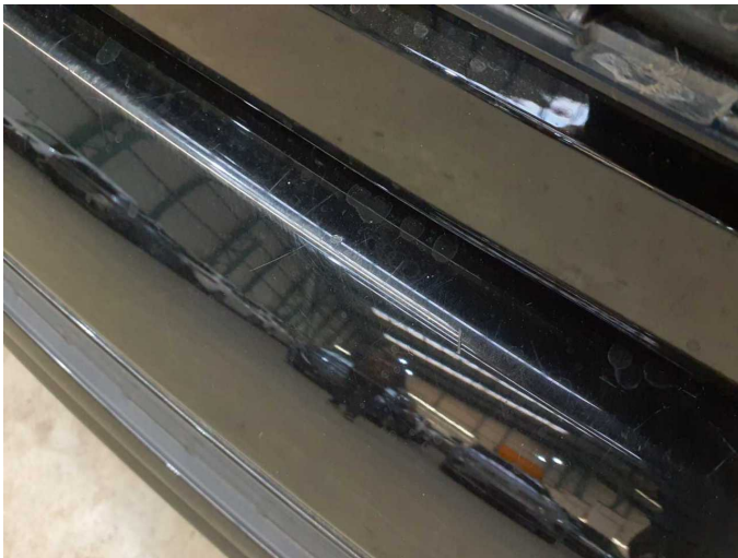
Damage 5: Rear bumper: Rear bumper - Scratch(es) - Paint
