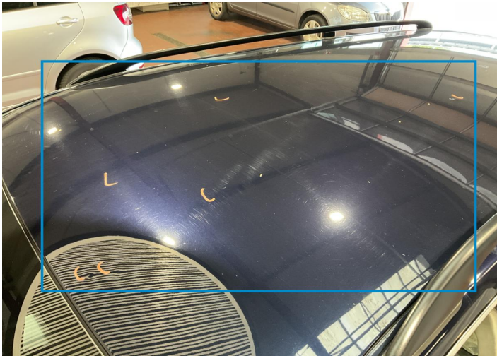
3. Roof Bodywork / Dent / Dent -
