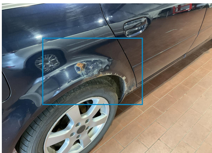
11. Side Panel / Back Right Paint / Corrosion -
