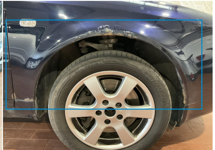
14. Fender / Front Right Paint / Corrosion -
