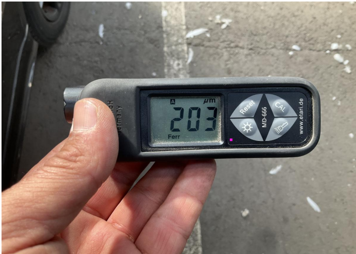
7. Door / Back Left Paint / Poor Previous Repair -
