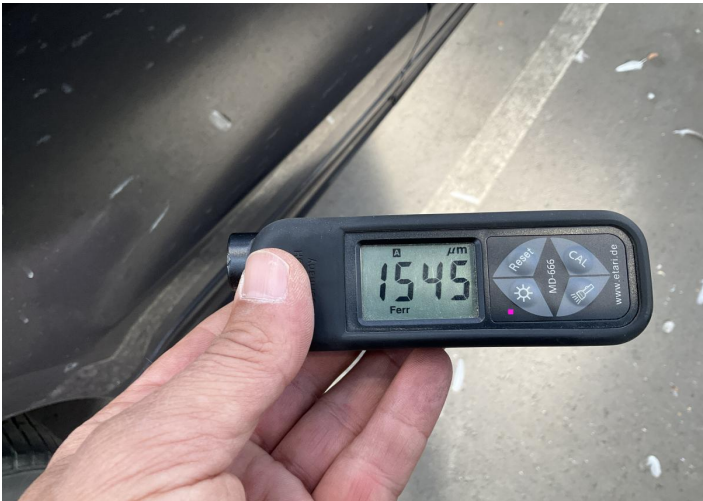
8. Door / Back Right Paint / Poor Previous Repair -
