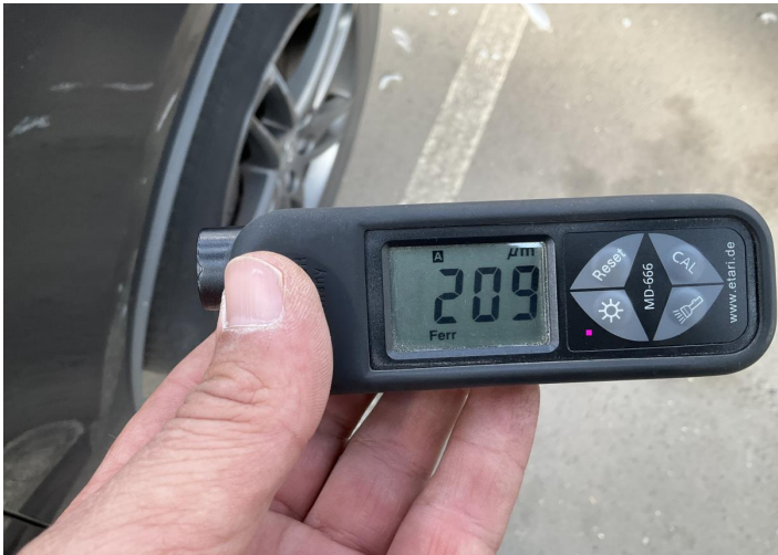
9. Door / Front Right Paint / Poor Previous Repair -
