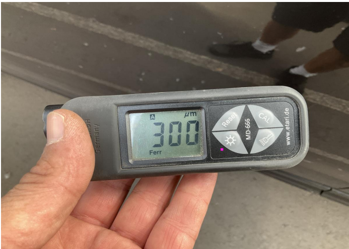
6. Door / Front Left Paint / Poor Previous Repair -
