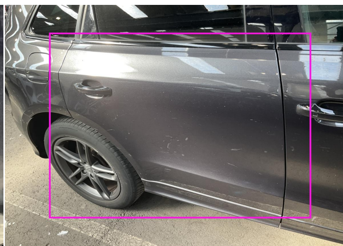
22. Door / Back Right Bodywork / Dent / Dent -
