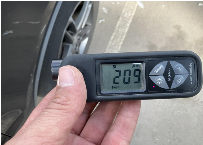
9. Door / Front Right Paint / Poor Previous Repair -
