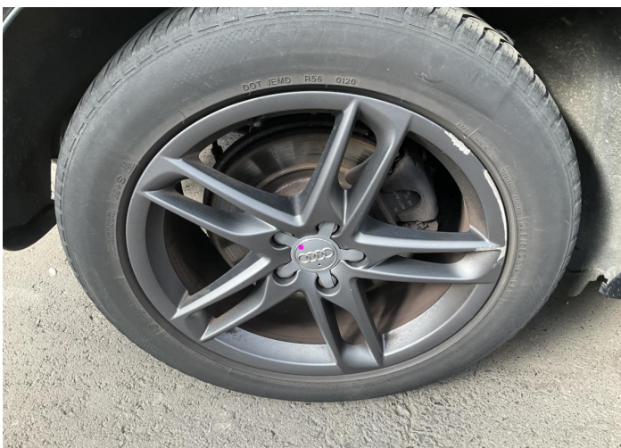
18. Rim / Back Right Out of Bodywork / Scratch -
