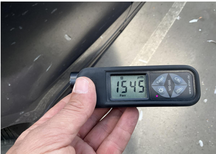
8. Door / Back Right Paint / Poor Previous Repair -
