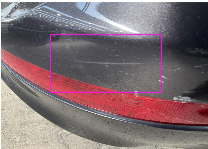
17. Corner Bumper / Back Right Paint / Scratch / Scuff -
