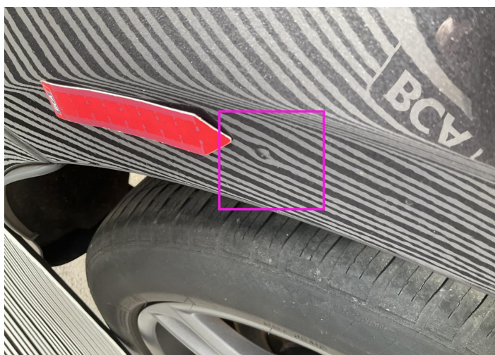
19. Side Panel / Back Right Bodywork / Dent / Dent -
