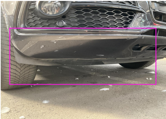
11. Corner Bumper / Front Right Paint / Scratch / Scuff -
