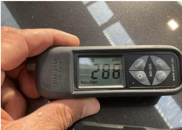
5. Hood Paint / Poor Previous Repair -
