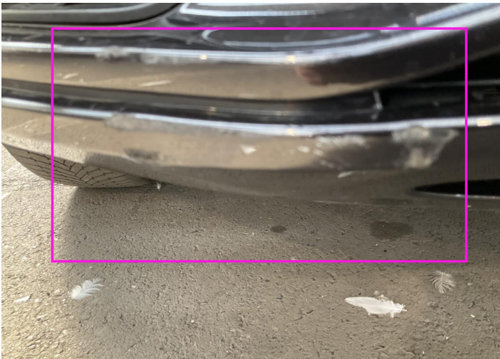
12. Corner Bumper / Front Right Bodywork / Dent / Dent -
