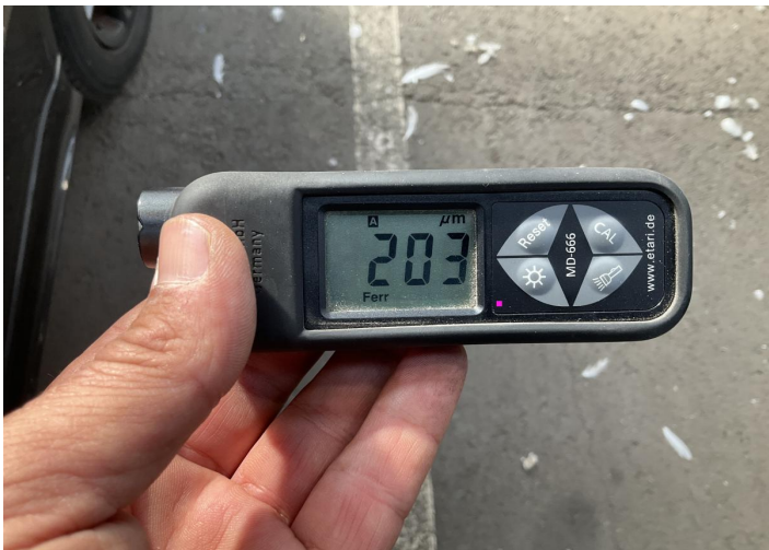
7. Door / Back Left Paint / Poor Previous Repair -
