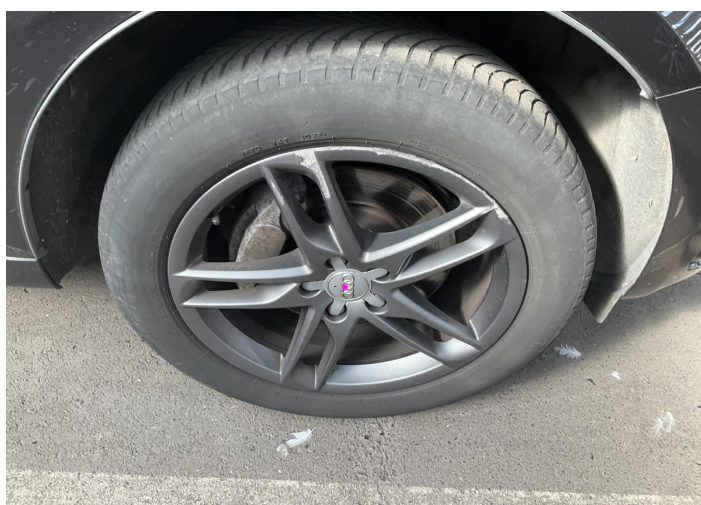
23. Rim / Front Right Out of Bodywork / Scratch -
