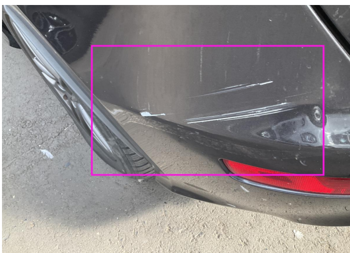
15. Corner Bumper / Back Left Paint / Scratch / Scuff -
