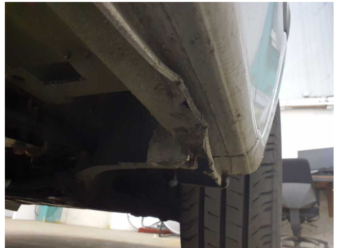
Damage 3: Sill - right side: Sill - Damaged - Repair and paint
