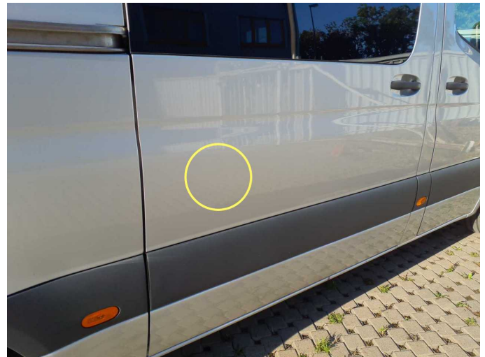
Damage 1: Sliding door, right: Sliding door - dent(s) - Smooth repair work
