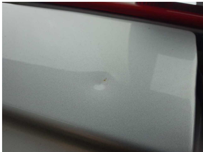
Damage 4: Boot lid / rear door: Rear door - left side - Dent / paintcoat damage - Repair and paint
