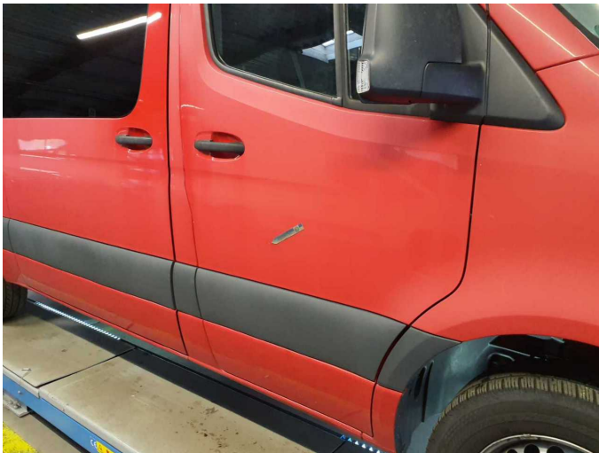
Damage 4: Door - front right side: Door - Scratched - Smart repair
