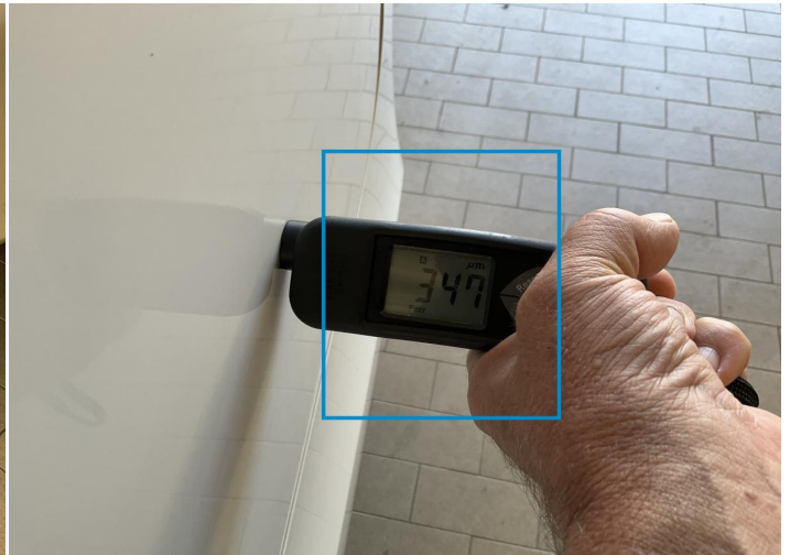
8. Side Panel / Back Left Paint / Poor Previous Repair -
