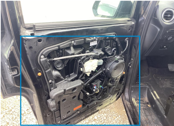
1. Panel Filling / Front Left Interior / Missing -
