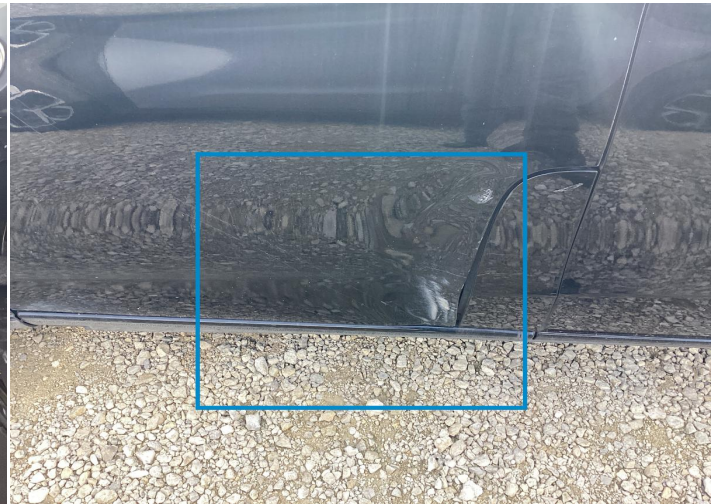
2. Door / Front Left Bodywork / Dent / Deformation -
