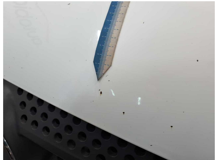
Damage 8: Bonnet: Bonnet (+Korrosion) - Stone chips - Paint
