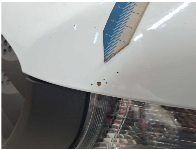
Damage 8: Bonnet: Bonnet (+Korrosion) - Stone chips - Paint
