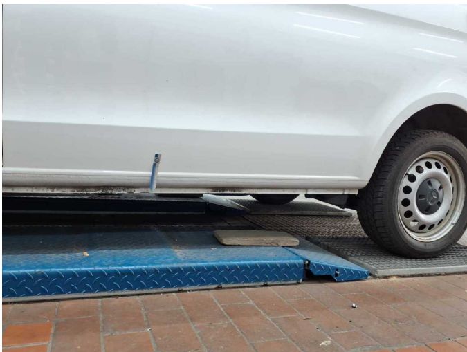
Damage 2: Sill - left side: Sill - Deformed - Loss in value
