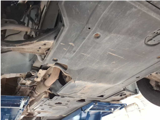
Damage 5: Body: Underbody panelling - Broken / torn - Replace
