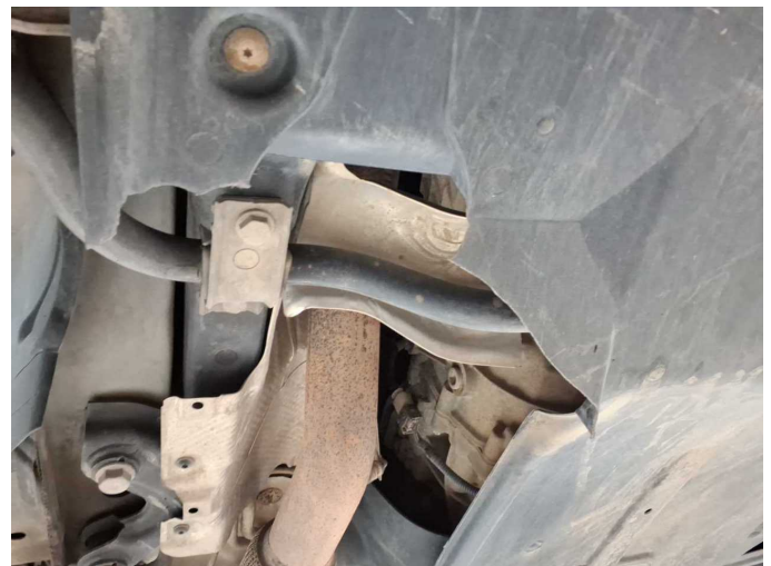
Damage 5: Body: Underbody panelling - Broken / torn - Replace
