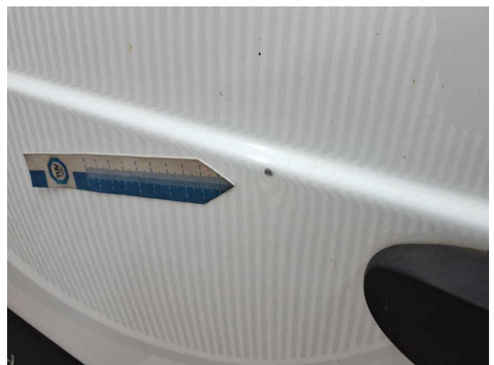
Wear and tear 5: Boot lid / rear door: Rear door - left side - Dent / paintcoat damage - No deduction
