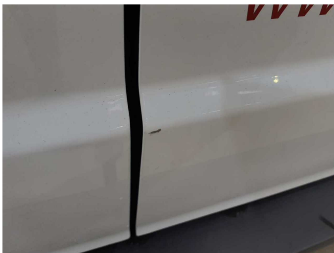
Damage 3: Boot lid / rear door: Rear door - right side - Dent / paintcoat damage - Repair and paint
