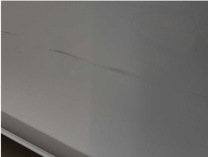
Damage 6: Sliding door, right: Sliding door - Scratch(es) - Paint
