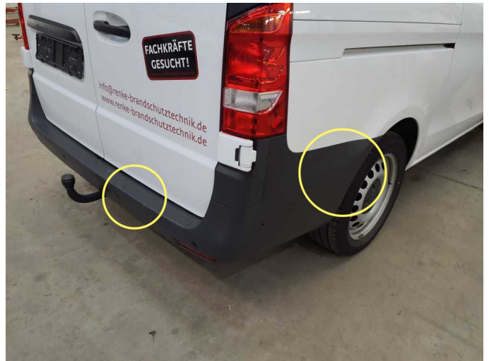
Damage 1: Rear bumper: Rear bumper (unpainted) - Scratched - Loss in value
