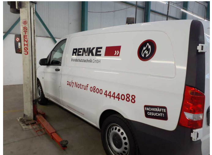
Damage 2: Body: Body - Glued / labelled - De-glue / neutralise
