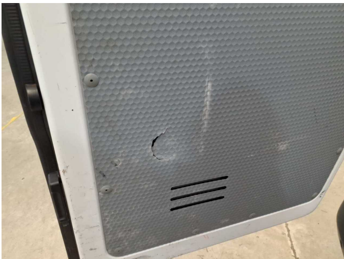
Damage 1: Trim / covers: Boot lid - interior trim - Broken / torn - Replace
